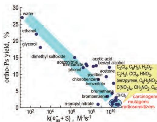
Figure 2. *o*-Ps yields (in %) in chemical compounds, S, vs. their reaction rate constants,  $k(e^- + S) M^{-1}s^{-1}$ , with hydrated electrons,  $e_{aq}^-$ . The chemicals were not dissolved in a solvent, but were taken "as is" (as a monophasic substance).
