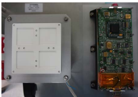
Figure 7. Mercury Dust Monitor (MDM) on-board BepiColombo MMO, which is composed of PZT piezo ceramic detector (40 mm × 40 mm × t2 mm × 4 pieces) coated with white paint reflecting the solar light, and electronics.
