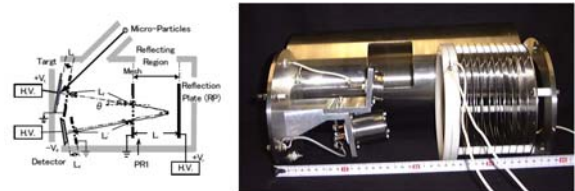
Figure 11. Schematic diagram of a reflection type Time-Of-Flight (TOF) mass spectrometer and a photograph of a prototype instrument.
