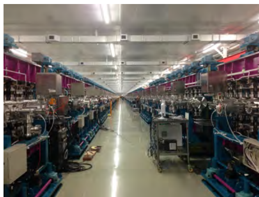
Photo 2. Two 90-meter long in-vacuum undulators of SACLA X-ray free electron laser facility.
