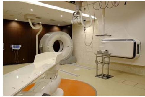
Figure 9. Commissioning setup in the treatment room; The QA phantom located on the front of the irradiation port is used for the commissioning of the patient positioning system and the irradiation system.
