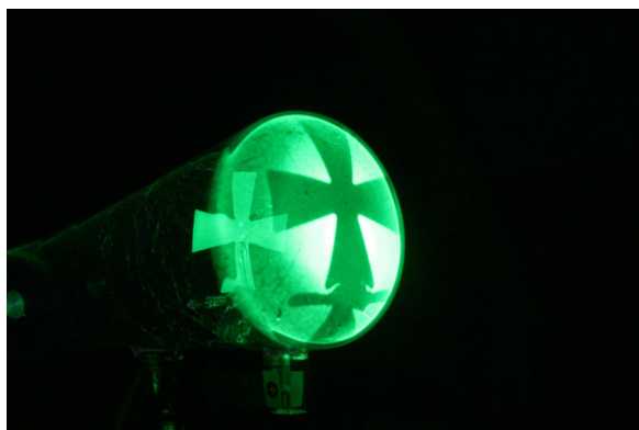
Figure 1. A Crookes tube in operation with a Maltese cross plate.
