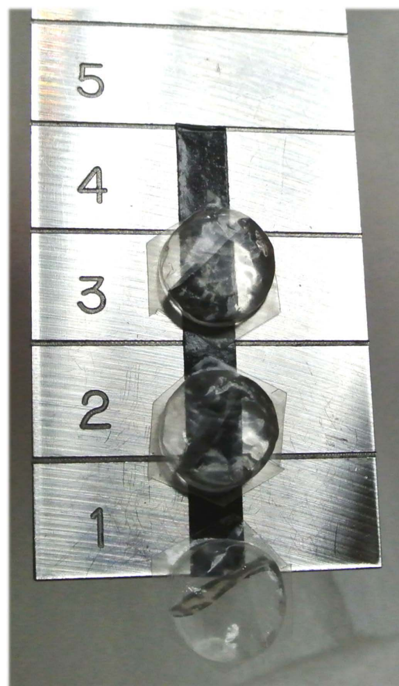
Figure 3. Photographic view of sample holder and bubble wraps for liquid sample. These bubble wraps are fixed with double-sided tape on the holder.
