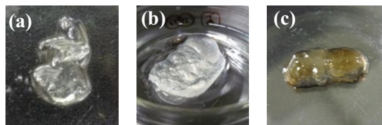
Figure 2. Photographs of radiation crosslinking (a) cellulose, (b) chitin, and (c) chitosan gel in ionic liquids.
